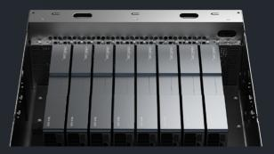
ATOM™-Max Server is a power-efficient, single-server solution built for large-scale Al inference. It supports up to 8 ATOM™-Max PCle cards, enabling deployment of hundreds of Al models spanning Vision Al, LLMs, Multimodal Al, and even Physical Al workloads. Fully compatible with leading inference frameworks like vLLM, Triton, and Kubernetes, you can seamlessly transition from GPU workflows with familiar tools and guided tutorials.
